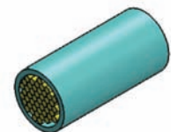
Duct containing 48 x Ø 1.2mm cable
